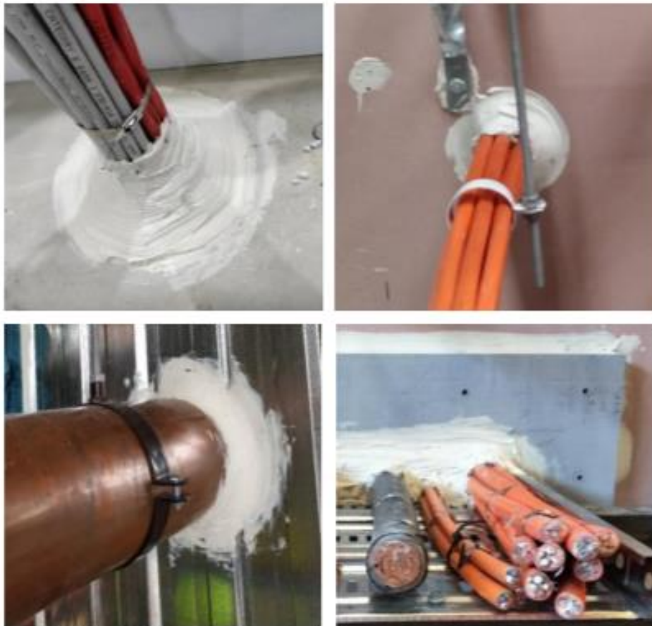
Penetrations tested in Hebel, SPEEDPANEL, FyreBOARD Maxilite, Plasterboard and concrete fire barriers
