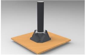
Select the correct size CIPEX Cast-in collar. The collar is nailed to the formwork, with a section of PEX-AL-PEX pipe installed through the collar extending above the planned slab level to form the penetration.
