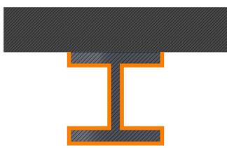
EXPOSURE CONDITIONS: I-section beam supporting lightweight or dense concrete slab.
