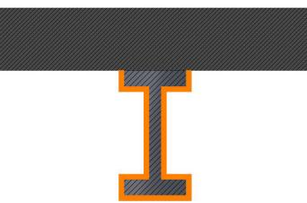
EXPOSURE CONDITIONS: I-section beam supporting lightweight or dense concrete slab.
