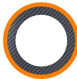
EXPOSURE CONDITIONS: Fully exposed steel beam or column sections. **Four (4) sided exposure. Critical temp: 550 deg. C. Ave.**
