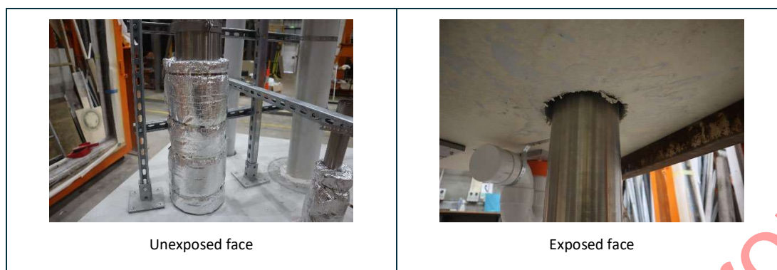
Specimen 7 – A Trafalgar Springbox – Blade with Pyrosafe DG cable bandage protecting a 100-mm diameter PVC pipe with floor waste incorporating a P-trap penetrating a 121-mm opening in the slab
