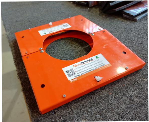
Floor waste applications are not continuous pipes, often having a metal grill finished at the floor level and a water trap installed below. The standard intumescent fire collars will not close off the penetration quickly enough to prevent early fire spread of fire through the floor grate, so a cast-in floor waste collar incorporating mechanical shutting mechanisms and are often specified to effectively close off the penetration, stopping the spread of fire in this unique application.
