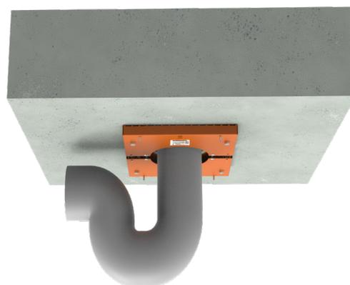
Place remaining half of the BladeRUNNER correct side up, with sticker exposed and visible, to the slab with the pipe between one half. Secure in the two holes in the BLADERUNNER using min. M6 x 50 masonry anchors. Care is to be taken not to overtighten the ancors. No sealant is required.
