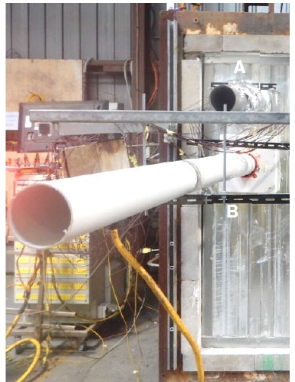
A photo of a fire test on a Trafalgar fire collar in a Speedpanel wall system
