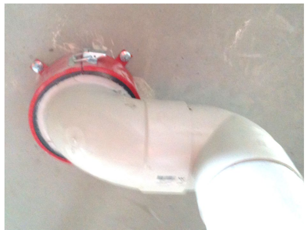
Fire collar with elbow inside collar before fire testing
