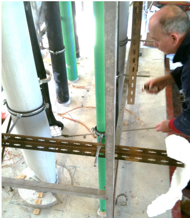
Different plastic pipes being fire tested with collars under the floor slab inside the fire test furnace
