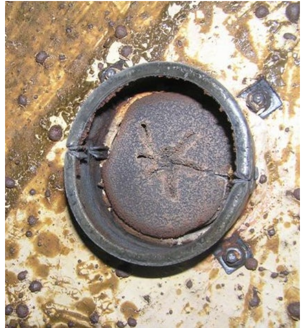
Photo of a Trafalgar Fire collar on the fire side after 4 hours of fire testing
