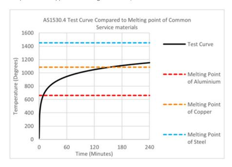
This means that for cable service penetration systems through fire rated barriers, we cannot directly apply previous cable testing from copper cables to aluminum cables because they will yield very different results. To address this, the National Construction Code (NCC) and AS1530.4 require that AL core cables should be tested separately to determine their performance as a penetration system.
