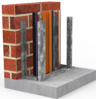
Frame the wall using 64mm steel studs at the perimeter and at 400mm centres. Use 6 x 45mm screws at 500mm centres. Fix framing to the surrounding walls and floors with appropriate fixings for the barrier.
