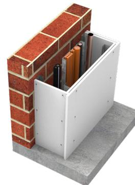
Apply the second layer of Trafalgar Corex board. Fix using Min 8g x 75mm plasterboard screws at 300mm centres.
