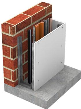
Apply the first layer of Trafalgar Corex board and fix using Min 8g x 45mm plasterboard screws at 400mm centres.
