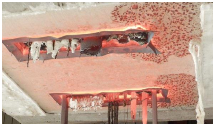
SuperSTOPPER® Cast-In after a 4 hour test.
