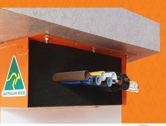
The FyreBOX™ Slab-Mount is a proudly Australian made passive fire penetration system used for multiple and mixed service penetrations which has been designed and tested to be built into residential/commercial apartment walls and riser shafts reducing the space required for service penetrations, providing predictable site costs and a reliable method of fire stopping.
