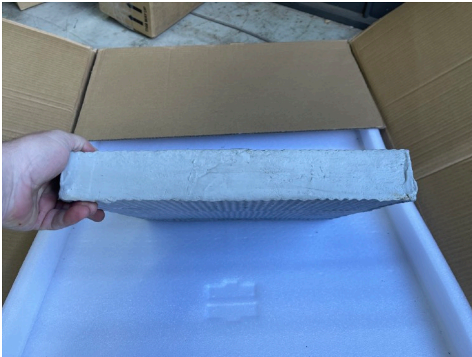
Ryanbatt 502 - no change after exposure - no corrosion
