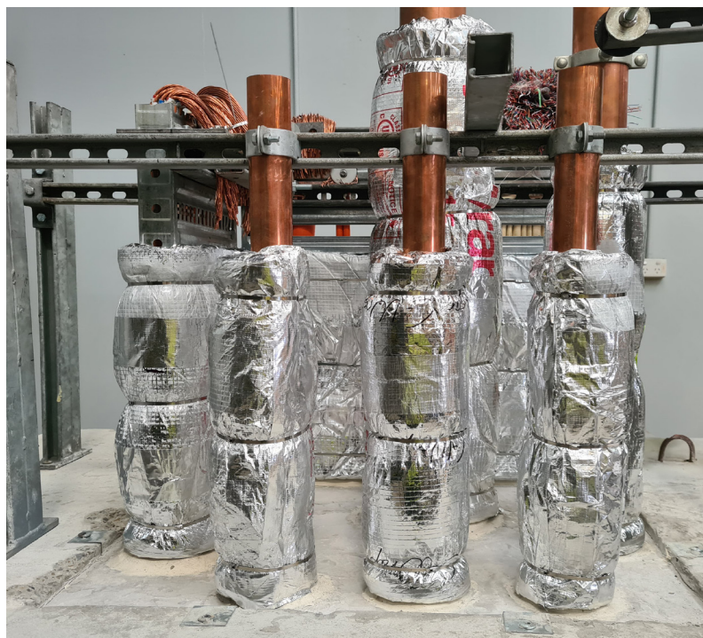
Image of an AS1530.4 fire test of our FyreSET® Mortar system being used in conjunction with FyreFLEX® and TWRAP™ to fire stop some copper pipes and cables.
