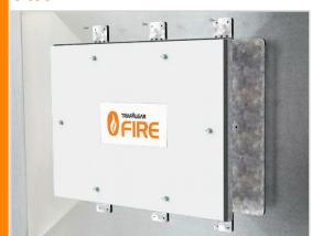
Using the preformed holes in the FWAP frame, drill and fix (using steel rivets or self-tapping screws only) the frame to the ductwork.
