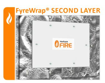
Install a second layer of FyreWrap® Elite 1.5, 100mm wide on all sides of the FyreWrap® Access Panel, fixing as per the standard FyreWrap® Elite 1.5 installation requirements (steel strapping or welded pins at 200mm centres).
