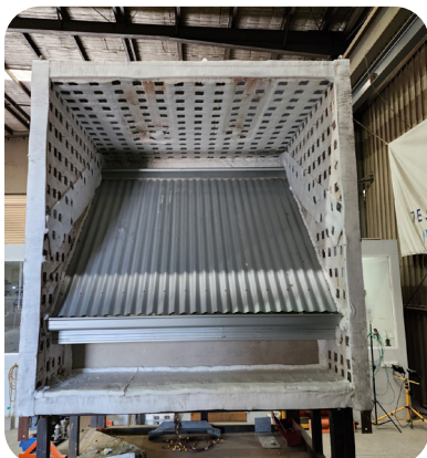
FyreROOF prior to AS1530.8.2 fire test
