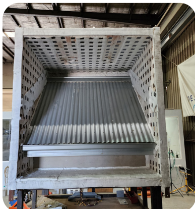
FyreROOF prior to AS1530.8.2 fire test
