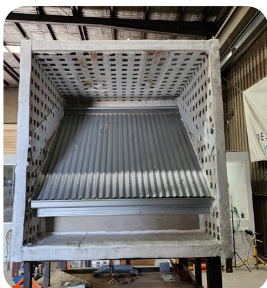
FyreROOF prior to AS1530.8.2 fire test
