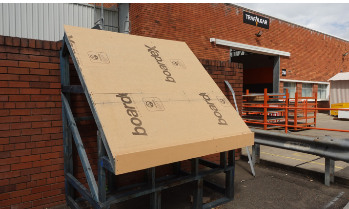
Trafalgar Boardex board being subjected to a weather test outside our Sydney Manufacturing Facility. The Board has remained in great condition over the last few years, despite harsh weather conditions. Visit our office to check it out!
