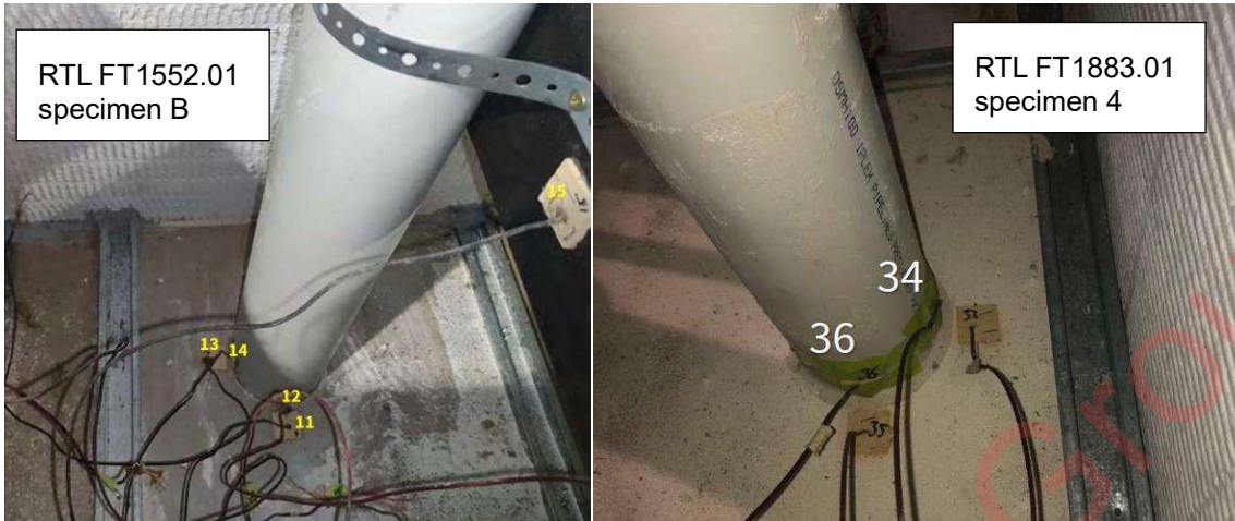
Figure 14 Thermocouples locations of the referenced tests
