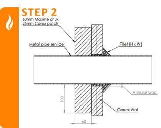
For stainless steel pipes, one side of the wall is required to be locally thickened for 100mm around the penetration with our 60mm thick FyreBOARD Maxilite® (or 3x layers of 25mm Corex board). Fix FyreBOARD Maxilite $^{TM}$  with min  $10g \times 100mm$  steel screws in each corner.
