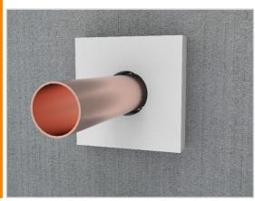
For 2 hour AAC walls (i.e. Hebel, Walsc), one side of the wall is required to be locally thickened for 100mm around the penetration with our 60mm thick FyreBOARD Maxilite®. Fix FyreBOARD Maxilite $^{\text{TM}}$  with min 10g x 100mm steel screws in each corner. Refer to page 31 for drawings. NOTE This is not required for -/90/90.
