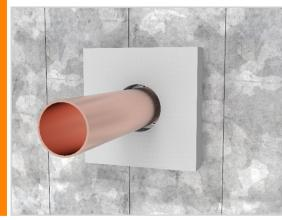
For Speedpanel®, one side of the wall is required to be locally thickened for 100mm around the penetration with our 60mm thick FyreBOARD Maxilite®. Fix FyreBOARD Maxilite™ with min 10g x 100mm steel screws in each corner. Refer to page 31 for drawings.
