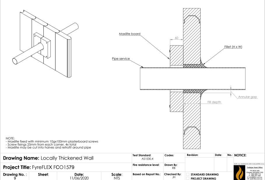
NOTE: Sealant drawing only (before wrap installation)
