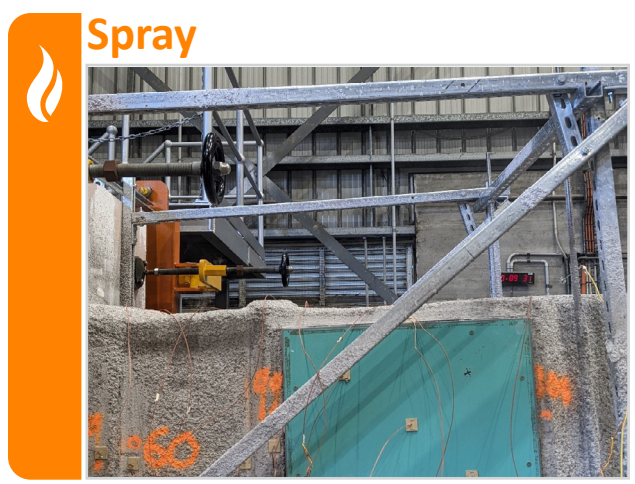
Spray as normal until the frame of the FDAP has been covered in spray for a width of 100mm.
