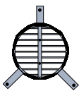
3 off fixing angles up to 250mm diameter 4 off fixing angles 300mm to 450mm diameter
