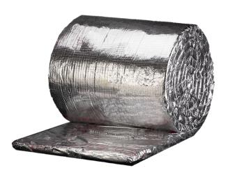
If required, TWRAP™ is wrapped around the services for the distance specified in the approval's tables. The TWRAP™ is to overlap itself by 50mm around the services at any joins, and is to be fixed with steel cable ties 50mm from each end and at 150mm centres between (or foil tape).
