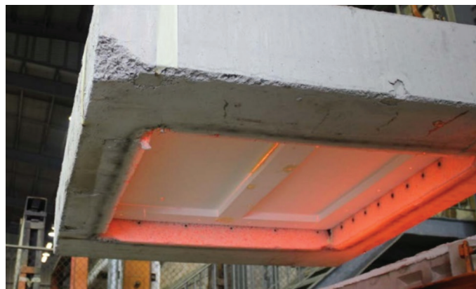
A calcium silicate board bulkhead system after being tested in a furnace to AS1530.4
