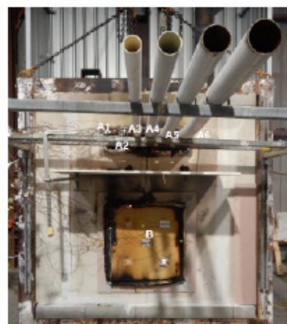
Figure 32 Unexposed face of the specimen at the end of the test
