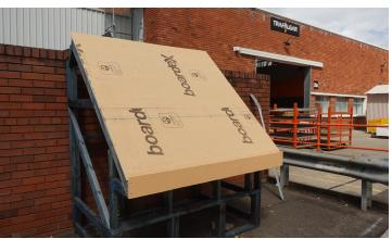
Trafalgar BoardeX board being subjected to a weather test outside our Sydney Manufactiring Facility. The Board has remained in great condition over the last few years, despite harsh weather conditions.
