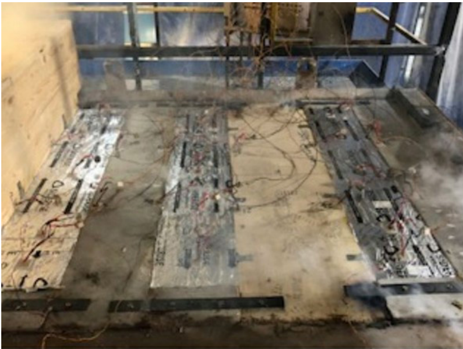
Here is an example of some SIDERISE cavity barriers undergoing AS1530 Part 4 exposure with CLT construction.
