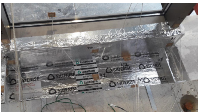
Fire tested to EN1364-4
