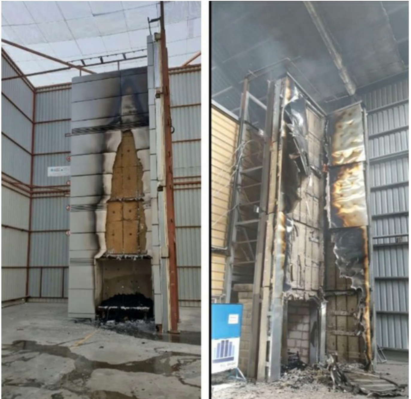
BS8414 Fire Testing of solid aluminium cladding with and without SIDERISE cavity barriers.
