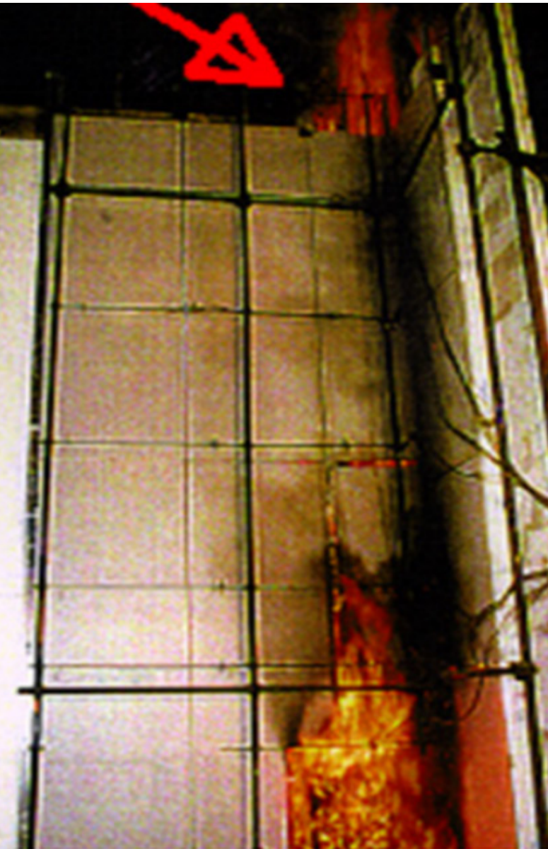
Fire Test with non-combustible fibre cement and Rockwool
