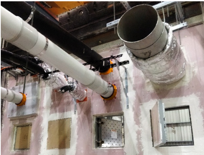
Image of an AS1530.4 fire test of various fire-stopping systems being used for a range of services.
